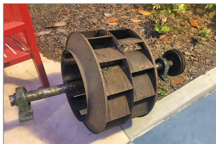
Old Blower Wheel Removed
